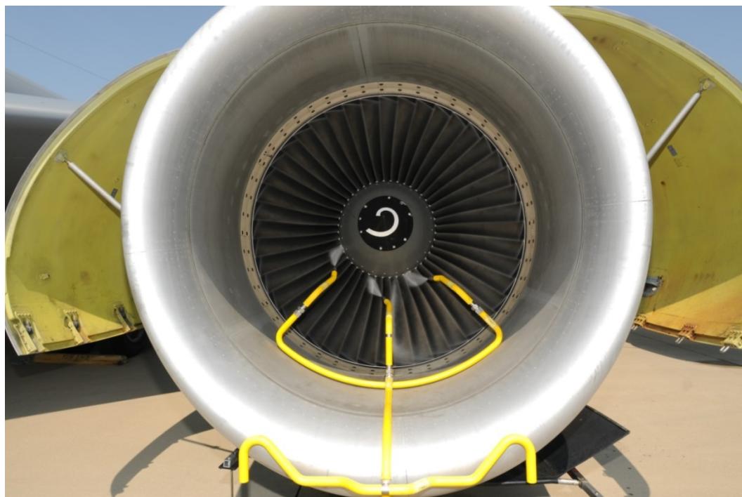
Figure 7c Engine Compressor Wash
